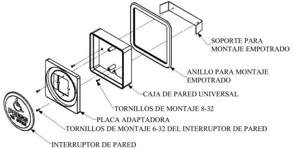
**INSTRUCCIONES DE MONTAJE DEL KIT DE MONTAJE EMPOTRADO**
